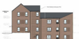
Block 1 Side Elevation (showing stepped levels arrangement)
